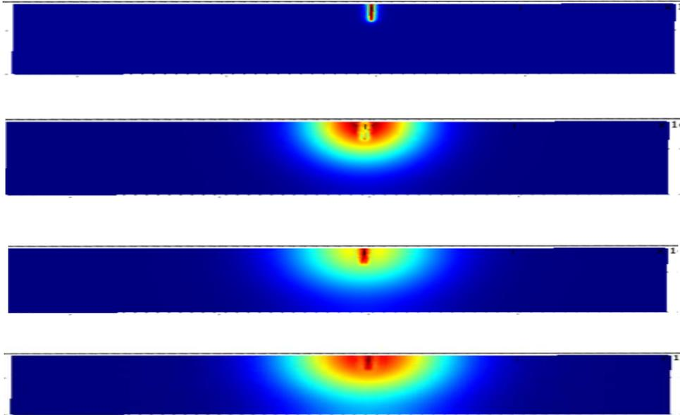
**Figure 6.** Numerical results of heat generation in plate with a crack, at different time steps. Heating is due to friction effect.
