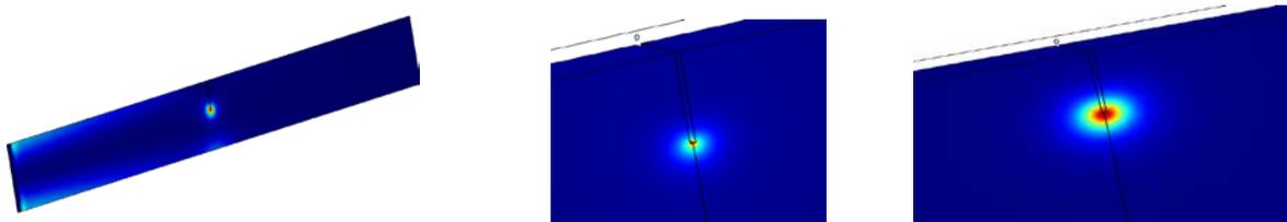
**Figure 3** Simulation results of heat generation for a damaged specimen
